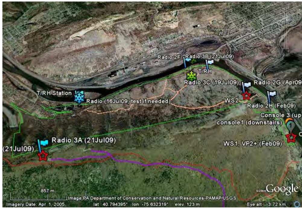
Overview of LGWR microclimate network (24 July 09) Flag=repeater radio, star=weather station, snowflake=T/RH station
