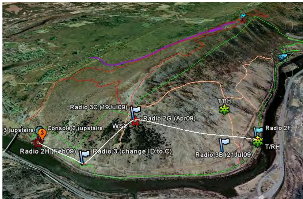
LGWR microclimate network 2, view from NE (24 July 09) Flag=repeater radio, star=weather station, snowflake=T/RH station, green line=LGWR boundary, red=AT, white line=radio path
